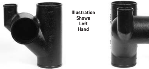
Part No. NH 457 Vented Closet Tee with 2" Top Vent (Left Hand or Right Hand; Designed for use below the floor; Fitting does not require a baffle.)
